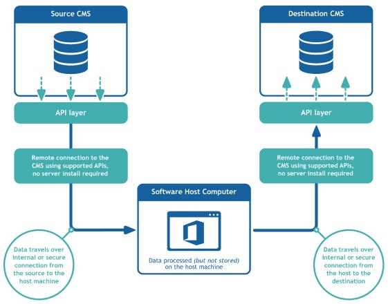
As we will discuss a little later, any obstacles or hurdles that sit in the process of this data flow (load balancers, firewalls, antivirus scanners, VPN, etc.) may have a negative impact on throughput. Wherever and whenever possible, we want to establish a path of least resistance.
