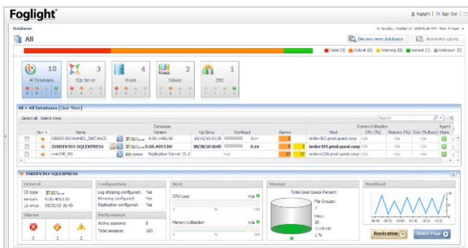
Foglight's global view provides one console for monitoring multiple database platforms, including DB2 LUW.
